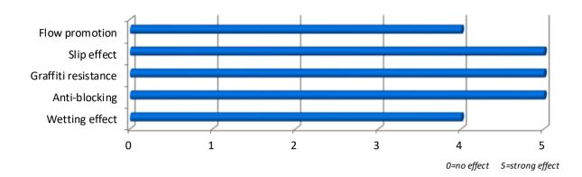
UNIQ FLOW 499 U is silicone surface additive. The additive can give excellent graffiti resistance of coatings after crosslinking because of the -OH group in it. UNIQ FLOW 499 U gives strong surface slip and excellent hand feelings. At the same time, it improves the anti-blocking properties.
